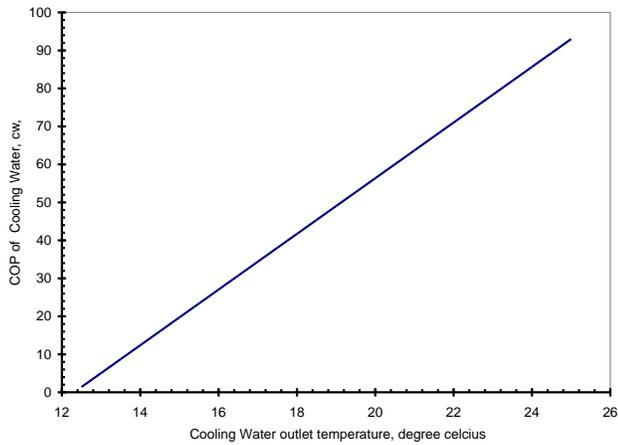
**Fig. 3.0 Plot of COP of Cooling Water against Cooling Water Outlet Temperature**
