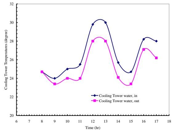
**Fig. 11.0 Plot of Cooling Tower Water Entry and Exit Temperatures against Local Time**
