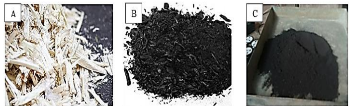
Figure 2 (a) Sugarcane-bagasse before burning (b) Sugarcane-bagasse after burning (c) Sugarcane-bagasse ash
