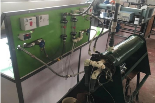
Figure 9: Experimental set up of CT50WS and Shell and Tube Heat Exchanger under load test condition.
