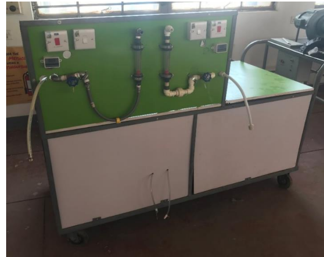
Figure 3: Constant Temperature Hot and Cold Water Supply System, CT50WS.
