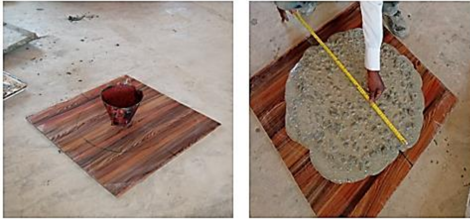
Figure 2: Slump flow of GCHA/WMPF concrete
