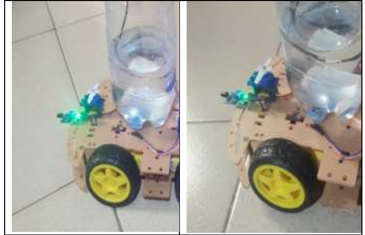
Figure 5: Complete diagram of the Autonomous Firefighting Robot
