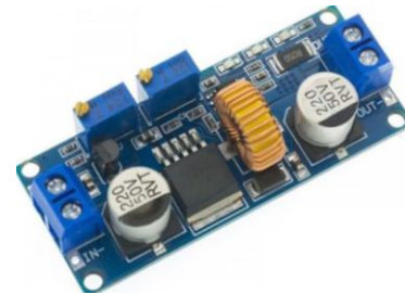
Figure 3: XL4015 5A Buck converter
