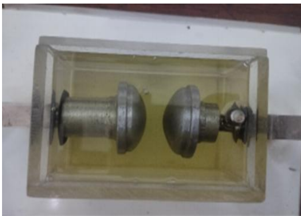
Figure 1 Mushroom – Mushroom Electrode Configuration
