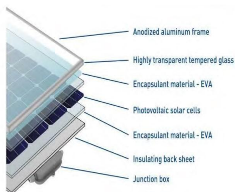
Figure 3: Structure of a PV Module (Sultan, et al. , 2019)
